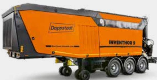
*“Our Inventhor series combines the best shredding technology from its predecessor, the renowned “Büffel” DW 3060, which has proven itself for decades, with the intelligent VarioDirect Drive concept. The separate setting of shaft and engine speed increases efficiency and possibilities by helping you to flexibly adapt the machine to your requirements.”*
