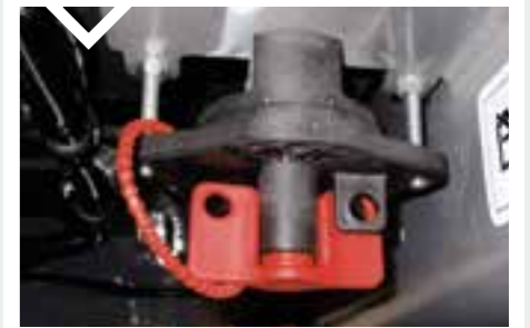
LOG-OUT TAG-OUT BATTERY MASTER SWITCH
