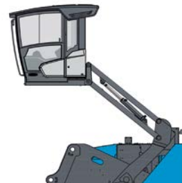
Cab system hydraulically adjustable
