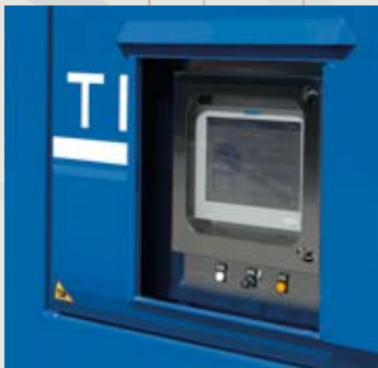
CHASSIS INTEGRATED ELECTRICAL PANEL
