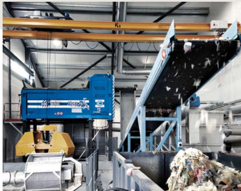
TIGER DEPACK HS 640 (FINLAND) / ORGANIC FRACTION OF URBAN SOLID WASTE FROM DIFFERENTIATED WASTE DISPOSAL
