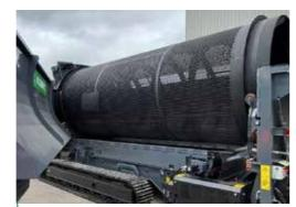
Easily replaceable 5.5m (18') x 2m (6'7") punch plate drum which is compatible with other manufacturers
