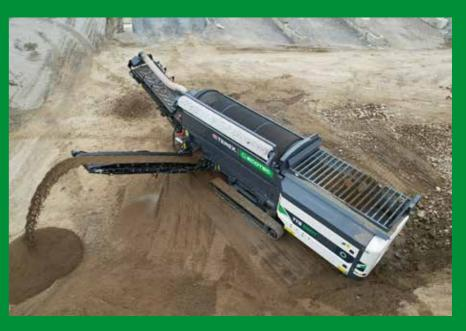
allows the operator to easily configure the machine to suit the required application. Whilst the intelligent feeder control system continually monitors the machine adjusting the feeder speed to optimise screening performance and throughput. Special consideration has been given to minimise the change out time for the screening drum. The process, which takes a matter of minutes, places the TTS 620 as a market leader.
