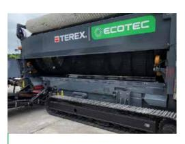
Double sided unrestricted drum access with low friction liners with access holes to combat material build up
