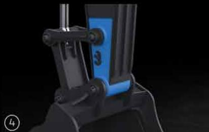
④ Reinforced casting tip
