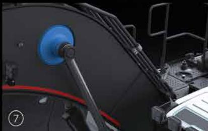
⑦ Reinforced boom cylinder cast bearing
