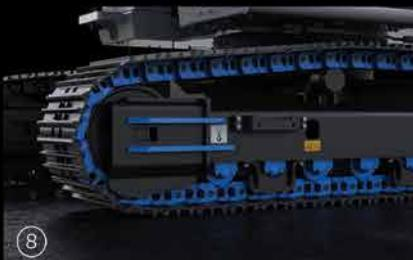
⑧ Reinforced lowerframe and undercarriage components
